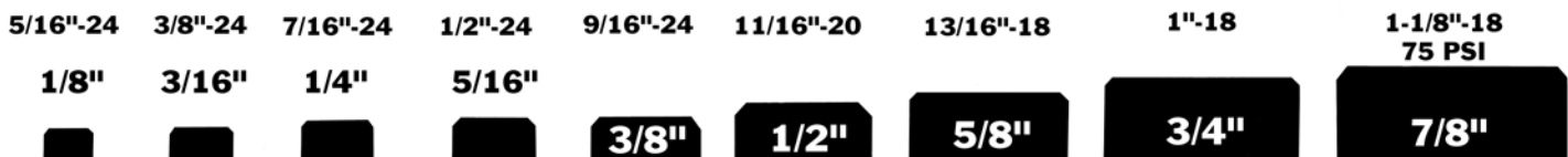
Actual Profile of Compression Threads
