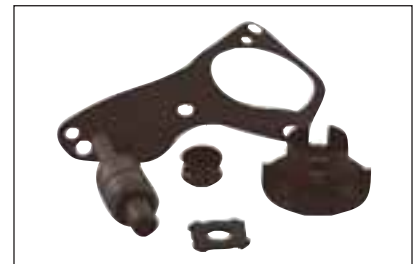
37-41 Water pump rebuild kit, trucks with double belt, passenger & commercial (2 kits required) . . . . . 79-8591 28.95 kit
