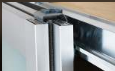
Sliding doors are opened and closed 20,000 times to test long-term functionality.
