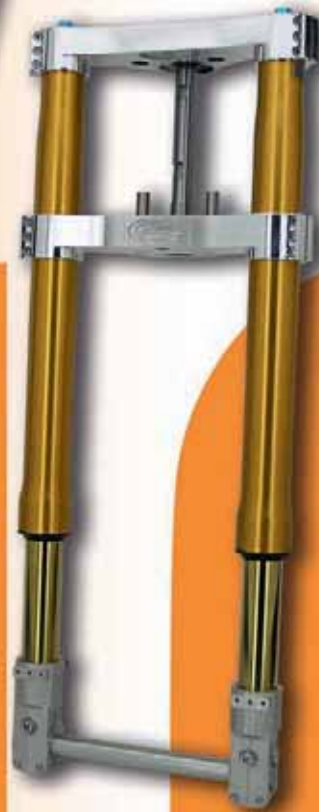
Rebuffini adjustable rake ladi triple trees
