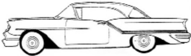
Holiday Coupe or 2 Door Hardtop. No post when door and rear quarter windows are rolled down.
