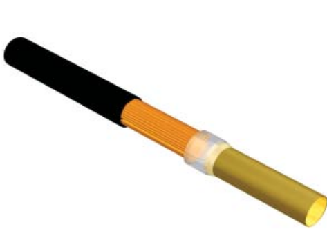
Wire is stripped and the appropriate size crimp sleeve is slid onto the strands.
