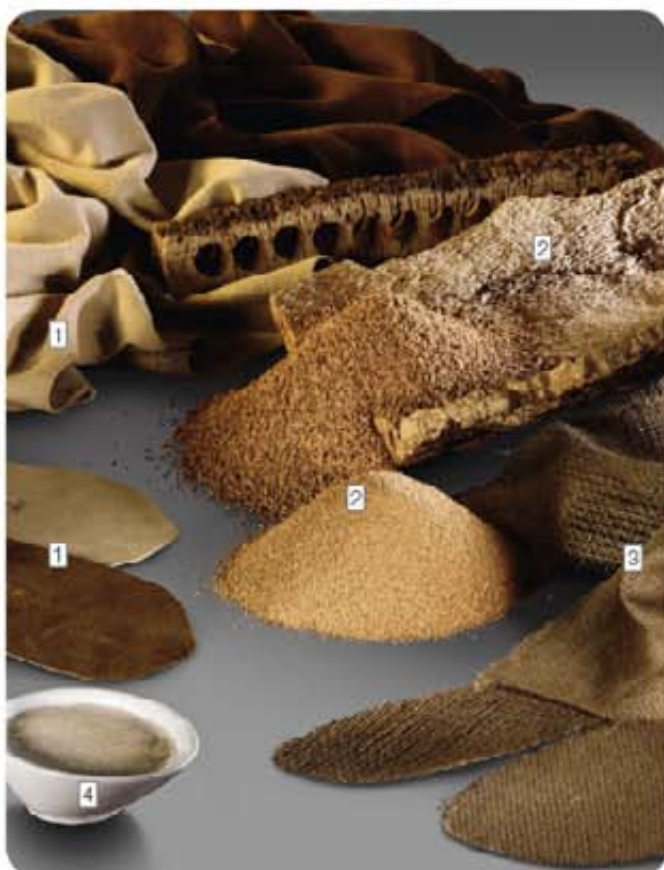
Suede leather in one piece and cut out (1), cork bark, stamping residue and granulate (2), fine and coarse jute (3) and latex milk (4) – natural materials for our footbed.
